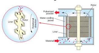
Super Rotor is equipped with a unique pulverizing rotor, which enables long-term stable and low-cost operation. Fine powder pulverization can be achieved without excessive pulverization. The pulverized particle distribution is very narrow.
