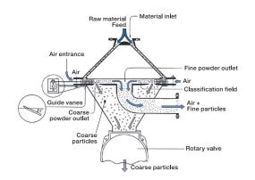
$\boldsymbol{\theta}$  degree inclined Guide vanes form the semi-free vortex, which best fit the coarse classification.
