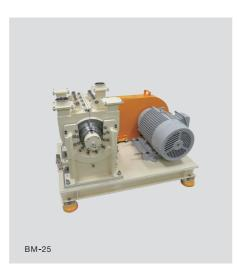
Because of a unique rotor blade structure, raw material, diameter at the micron level of up to several centimeters can be pulverized into powder with diameter of micron level.
